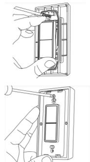
**NOTE:** For proper assembly, make sure to align the “top” labels on the rocker pad and wall plate.
