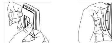
**TIP:** To remove the trim plate, use a flat-head screwdriver to depress the trim plate tabs using the 2 slots on the bottom of the wall plate. Alternatively, use a fingernail to press down along the top groove and flex the tabs out of the slots.
