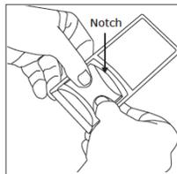
5. Hold both edges of the lens, flex it gently and push until it pops into the grooves. Make sure the edges are flush. NOTE: If the lens is out of position, the sensor will not detect activity properly.
