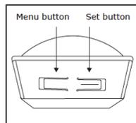
NOTE: The button interface on the sensor is used for linking and testing only. The occupancy timer settings are configured on the transceiver to which the sensor is linked.
