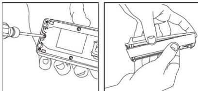
3. Remove the installed lens by gently squeezing it to ease one side out of its groove, and then the other.
