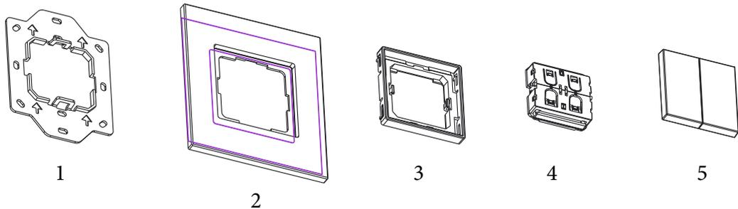
**WE SUGGEST MOUNTING ON A SOLID SURFACE:** Depending on the ground (brick plaster, glass...) the base plate can be glued or screwed. In any case, the ground must be smooth. Unevenness can lead to malfunctions! Watch that no dust is getting inside the housing.
